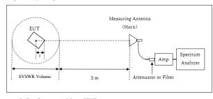
Distance Factor:  $20 \times \log (3.40 \text{ m}^*/3.0 \text{ m}) = 1.09 \text{ dB}$ \* Test Distance: (3 + SVSWR Volume /2) - r = 3.40 m
