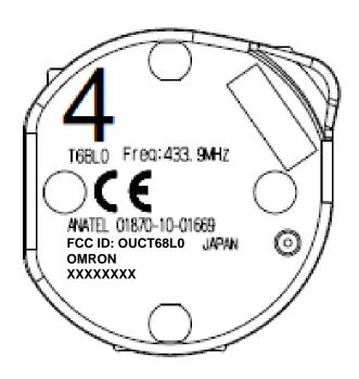
Figure 8.1 Label(marking) T68L0 appearance
