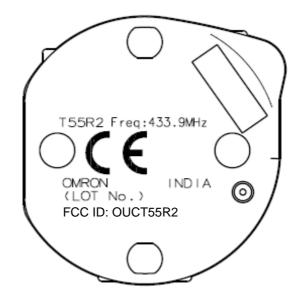
Figure 8.1 Label(marking) T55R2 appearance
