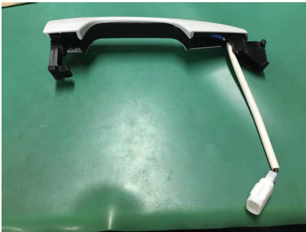
Figure 8.14 LF-antenna(Dr, As) appearance (back view)
