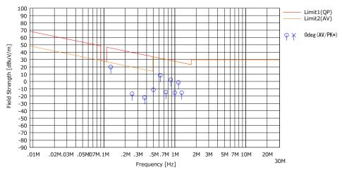
\* Data above 490 kHz were measured using a QP detector.
