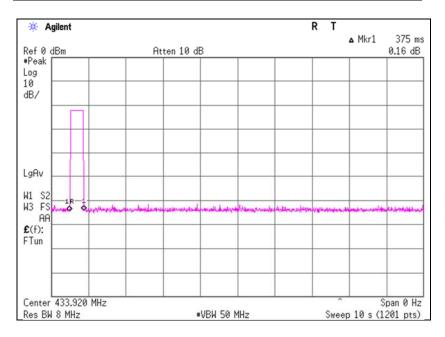
\* The EUT transmits UHF when LF signal is received from a car or a button on the EUT is pressed. In both cases, the UHF transmission is stopped within 5 seconds. So the test was performed by a button-pressed operation as the worst case.
