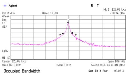
Jccupied Bandwidth 7.8102 kHz Occ BW % Pwr 99.00 % x dB -26.00 dB
