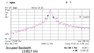
Transmit Freq Error 842.516 Hz x dB Bandwidth 20.065 kHz
