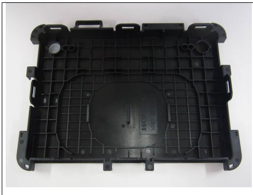
Figure 8.5 Cover Assembly [1] ~ [4] (bottom view)
