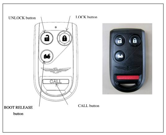
You can lock and unlock your vehicle with the remote transmitter.
