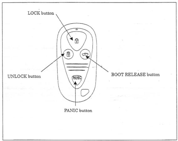
You can lock and unlock your vehicle with the remote transmitter.
