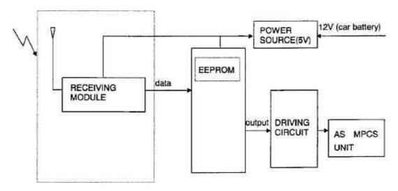
Figure 3.1 block diagram of the receiver
