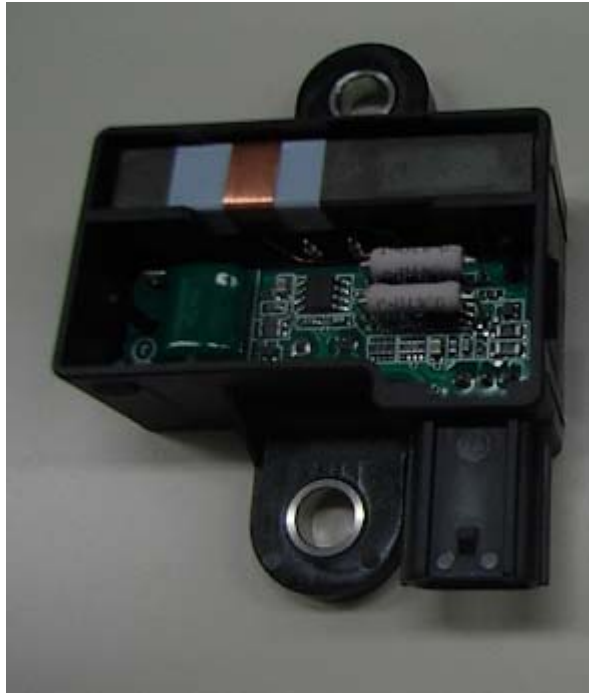
Figure 7.5 PCB assy and antenna ( inserted into case , front view)
