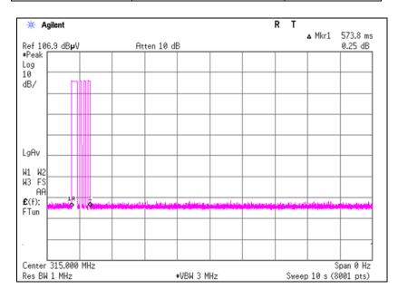
\* The EUT transmits UHF when LF signal is received from a car or a button on the EUT is pressed. In both cases, the UHF transmission is stopped within 5 seconds. So the test was performed by a button-pressed operation as the worst case. Please refer to the "Theory of operation".
