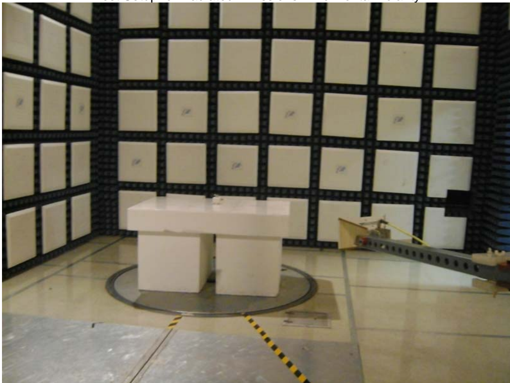
Test Setup for Radiated Emissions – Vertical Polarity
