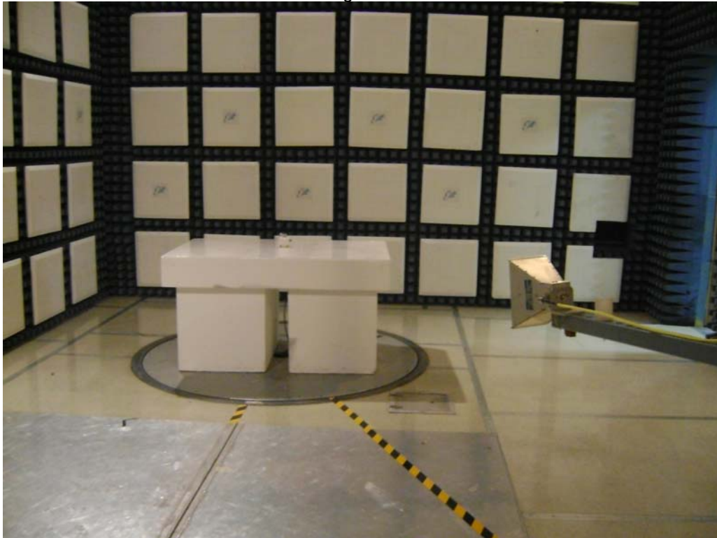
Test Setup for Radiated Emissions – Horizontal Polarity
