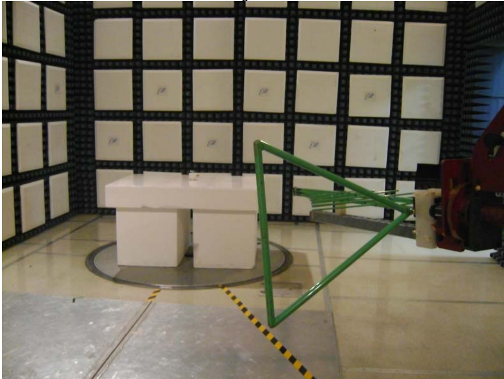
Test Setup for Radiated Emissions – Horizontal Polarity
