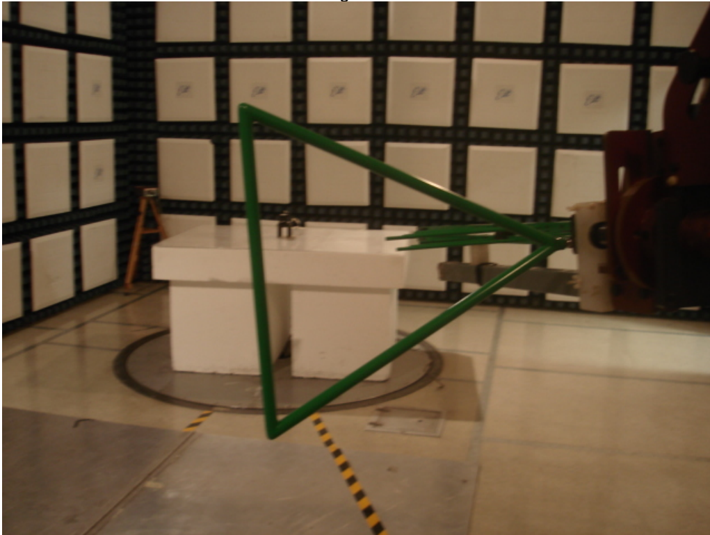
Test Set-up for Radiated Emissions – Horizontal Polarity
