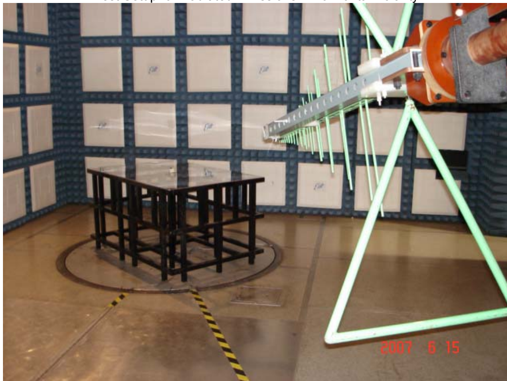
Test Setup for Radiated Emissions – Vertical Polarity
