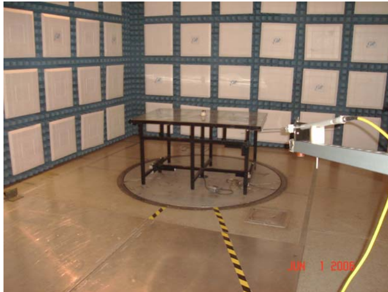
Test Set-up for Radiated Emissions Horizontal Polarity
