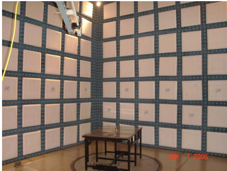
Test Set-up for Radiated Emissions Vertical Polarity
