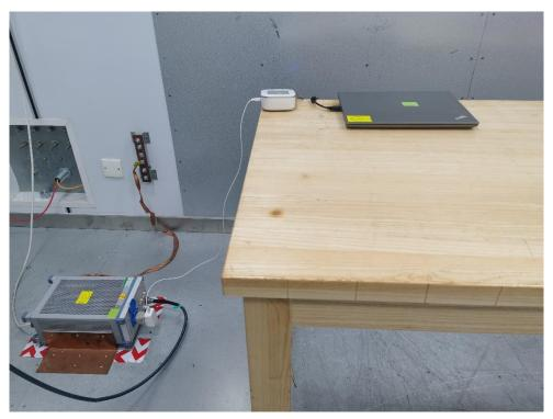
Radiated Disturbance below 1 GHz and above 30 MHz
