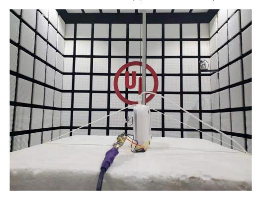
Radiated Disturbance Setup (Above 1 GHz - Z axis)
