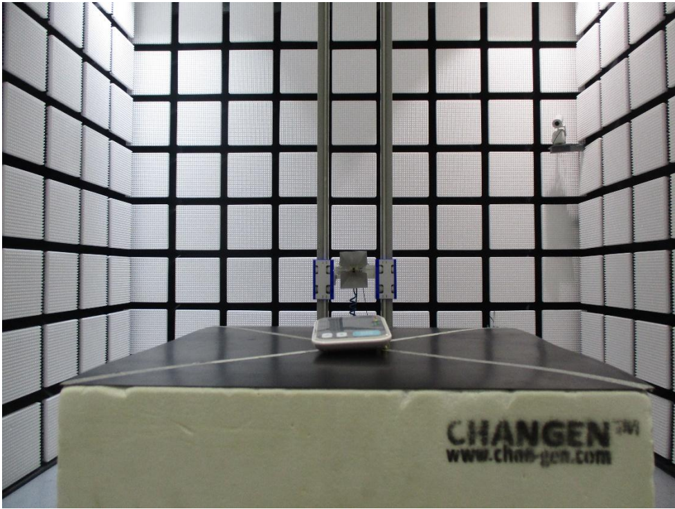
Radiated Emission Test above 1GHz
