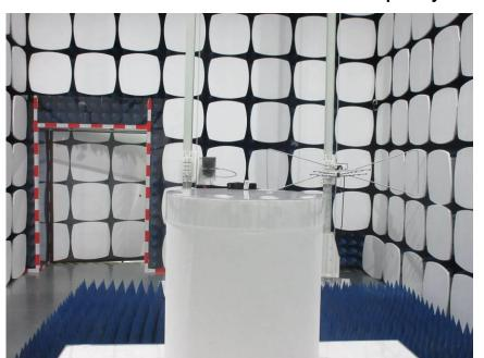
1.3 Restricted Band Around Fundamental Frequency Test Setup
