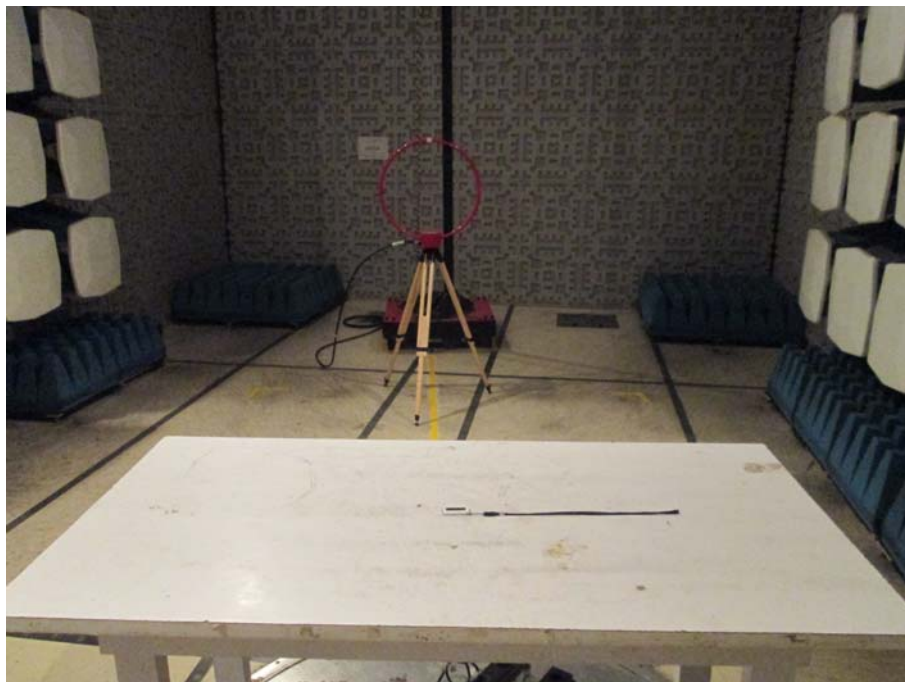
TEST SETUP OF RADIATED EMISSION-1
