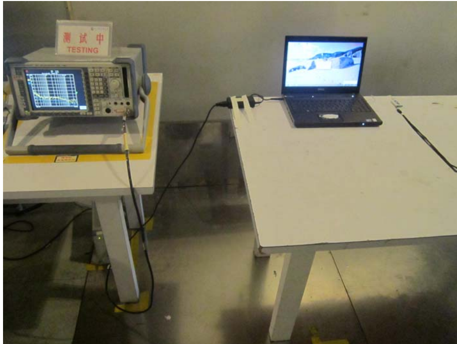
TEST SETUP OF CONDUCTED EMISSION
