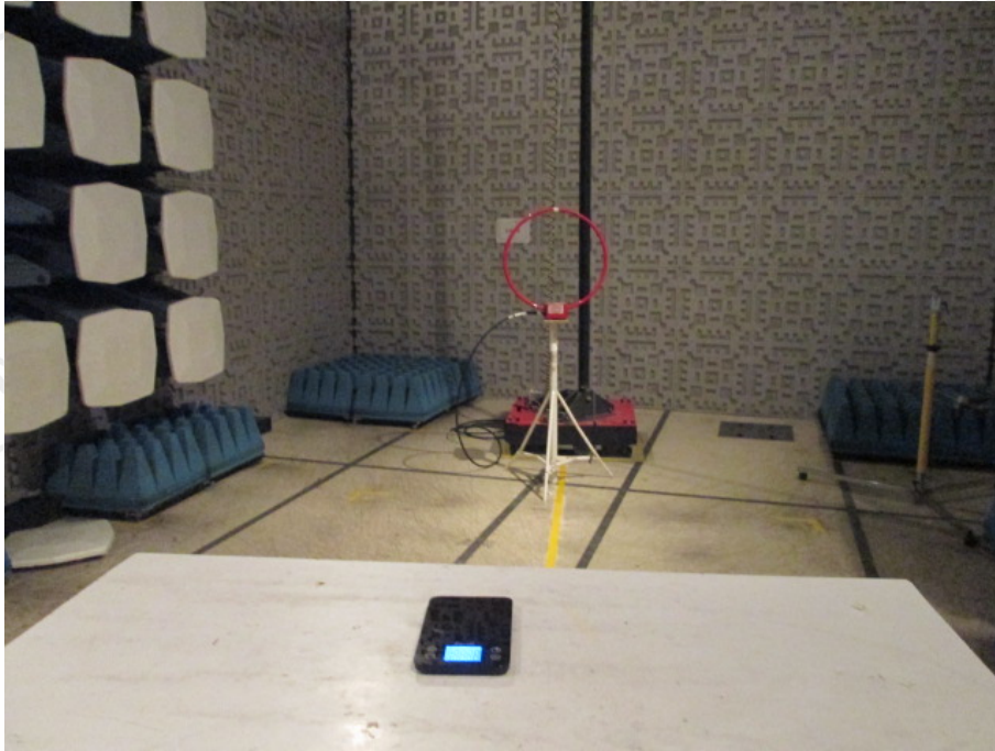
TEST SETUP OF RADIATED EMISSION-1
