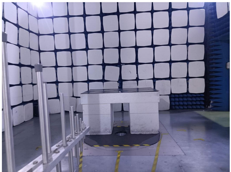
Radiation Emission Test Setup (30MHz to 1GHz)
