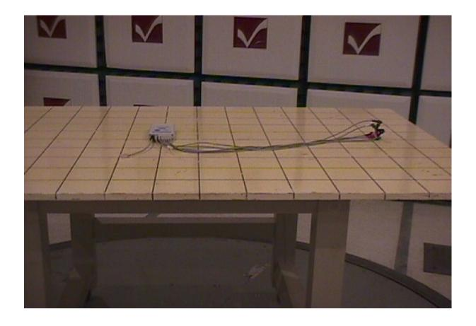
View of the Apex Pro transmitter during the Radiated Emissions tests. This view shows the orientation of the product corresponding to zero degrees azimuth in position. (horizontal polarity).
