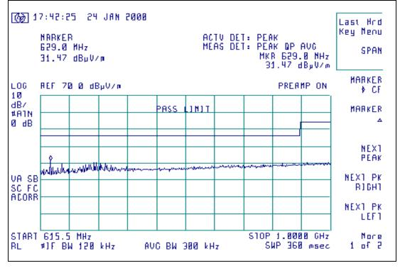
Radiated emissions, high channel (613.975 MHz), vertical polarity
