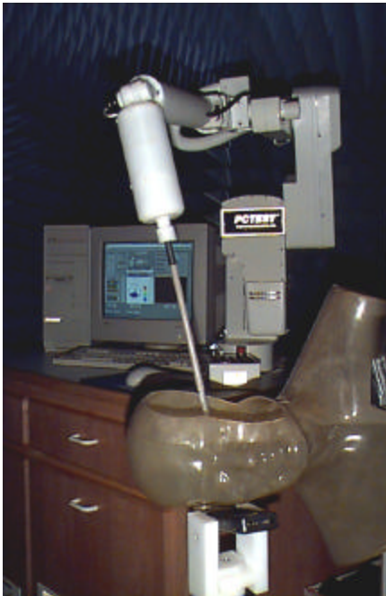
Figure 5. Photograph of the Probe and the Phantom
