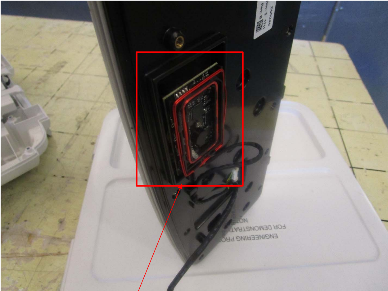
RFID radio OEM-805N2AKU is located behind the keyboard of the host
