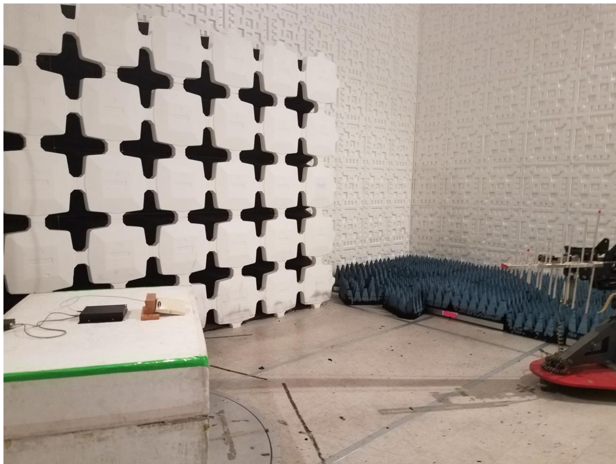
Figure 3. Radiated Emissions Test Setup, 200 MHz to 1GHz
