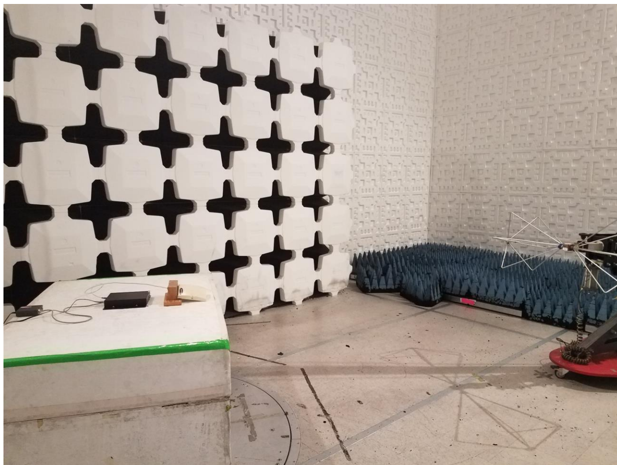
Figure 2. Radiated Emissions Test Setup, 30 MHz to 200 MHz
