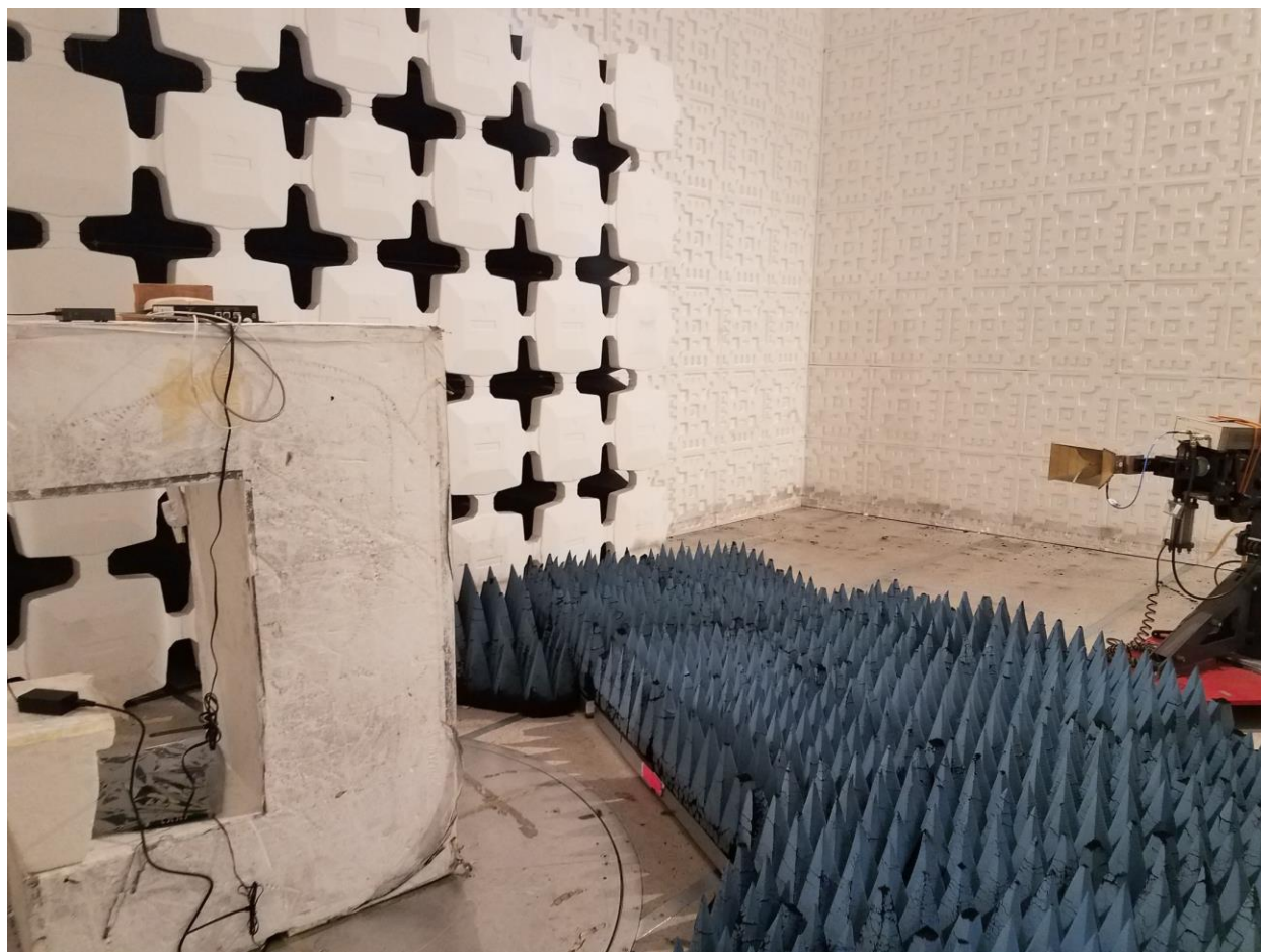
Figure 4. Radiated Emission Test Setup, above 1 GHz
