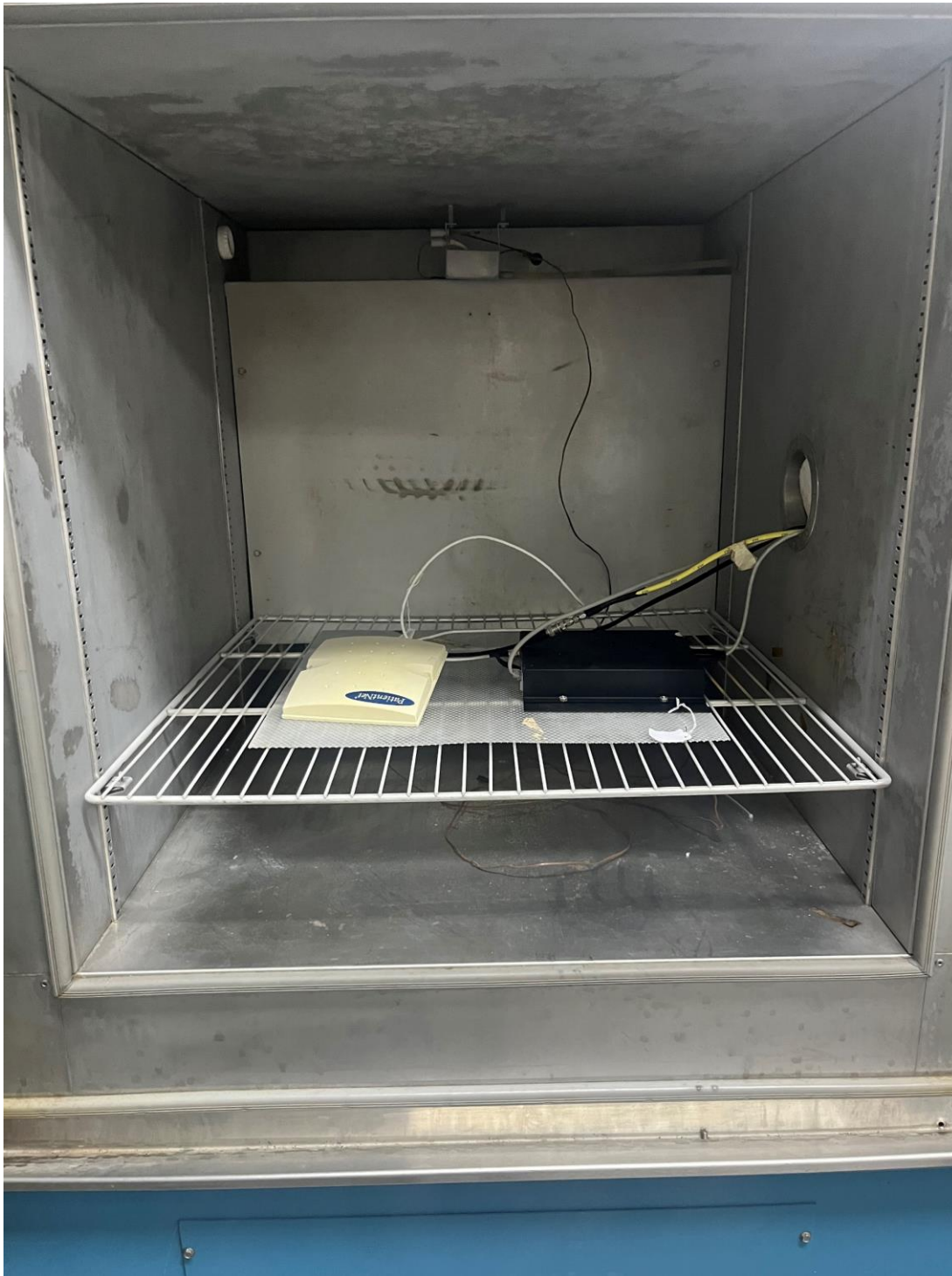
Figure 6. Frequency Stability Test Setup – Close Up
