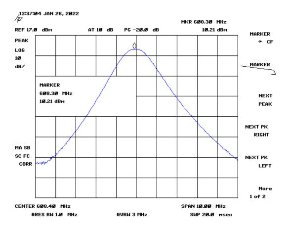
**Figure 6. Maximum Conducted Output Power**
