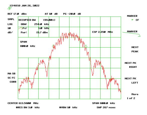
Figure 5. Bandwidth, High Channel
