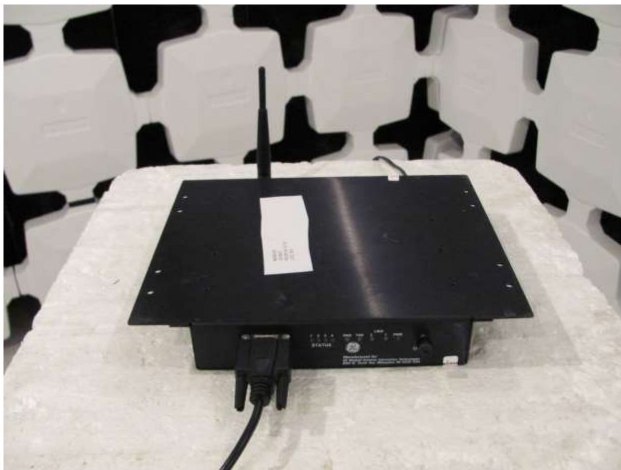
Figure 5. Radiated Emissions above 1 GHz, Dipole Antenna, Close-up Photo
