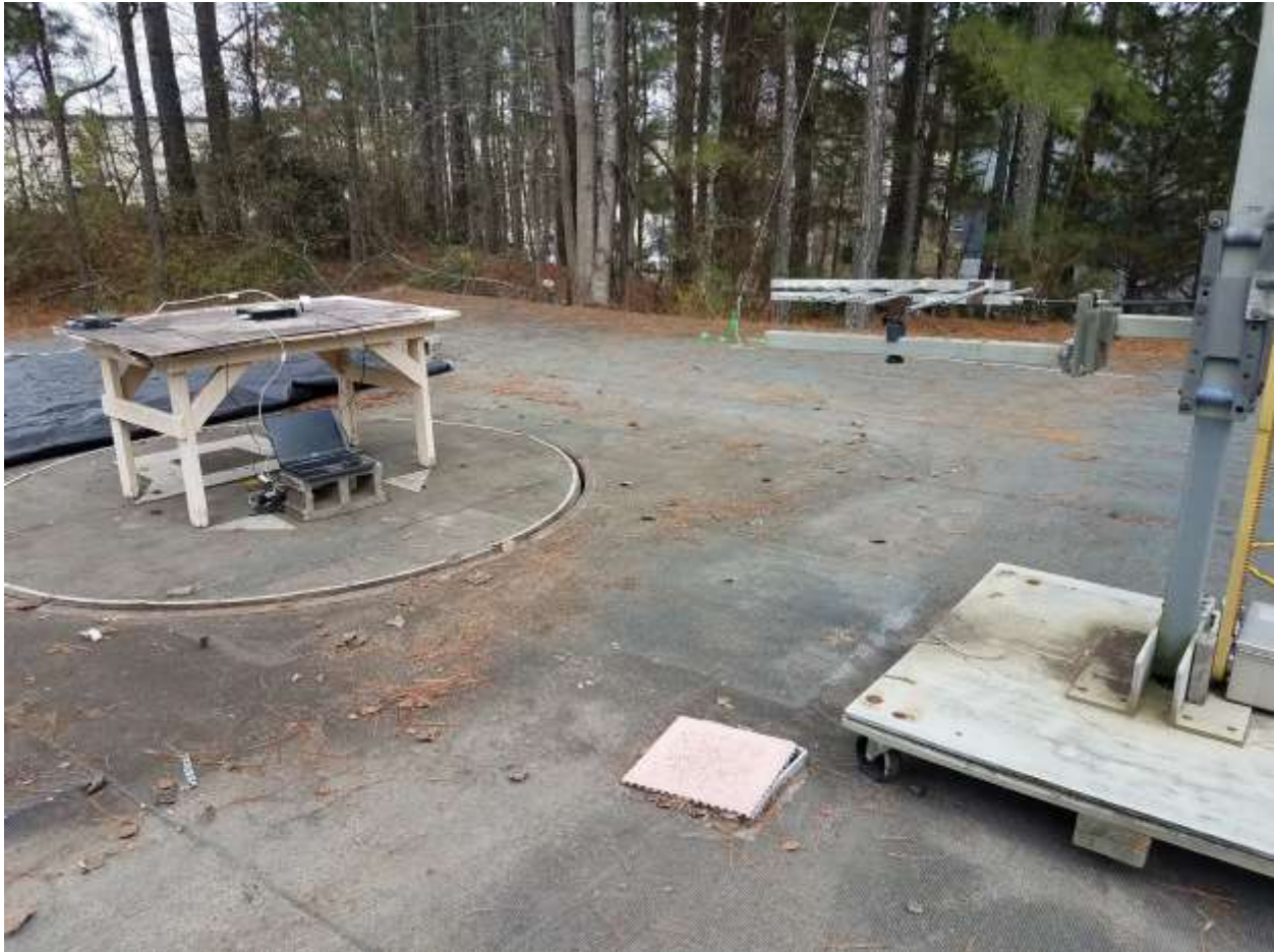
Figure 1. OATS- Fundamental measurement, Dipole (Antenna 1)
