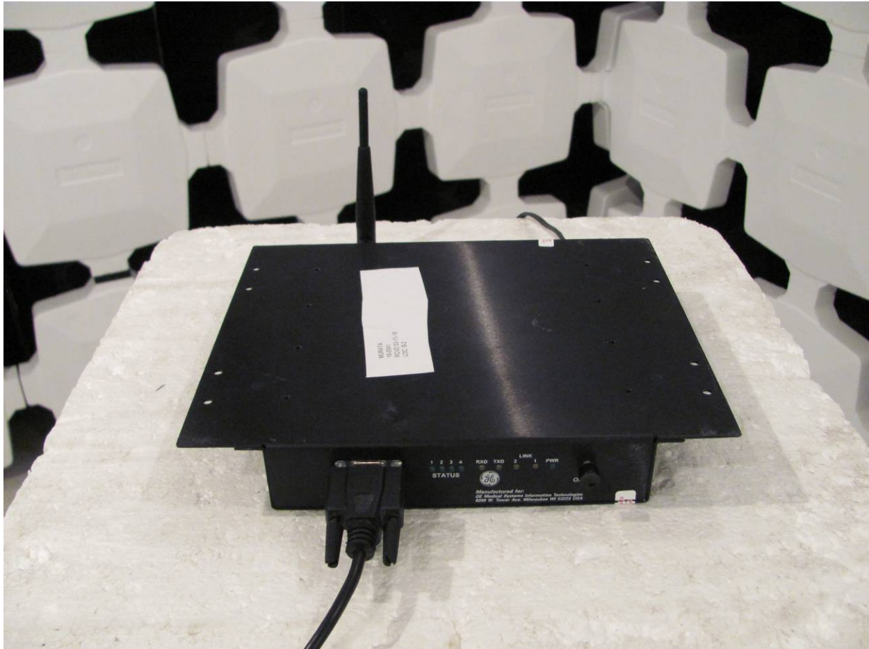
Figure 7. Radiated Emissions above 1 GHz (EUT placed on block elevated to 1.5 m test height)
