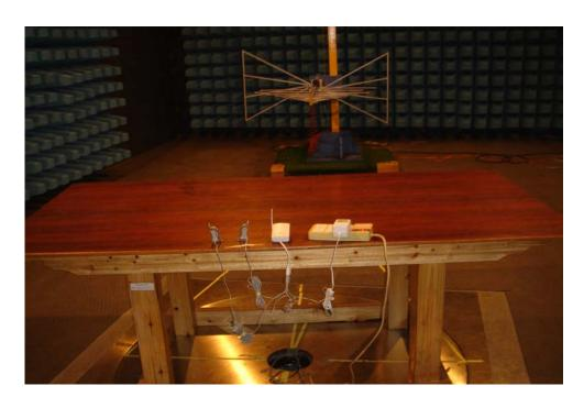
**Radiation Emission Test View For 1GHz-5GHz**
