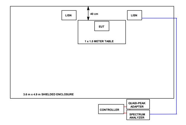
FIGURE 2: Radiated Emissions Test Setup
