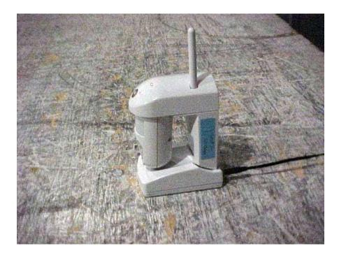
Xanboo Mcam XWC900 Security Camera Transmitter Radiated Emissions Test Setup
