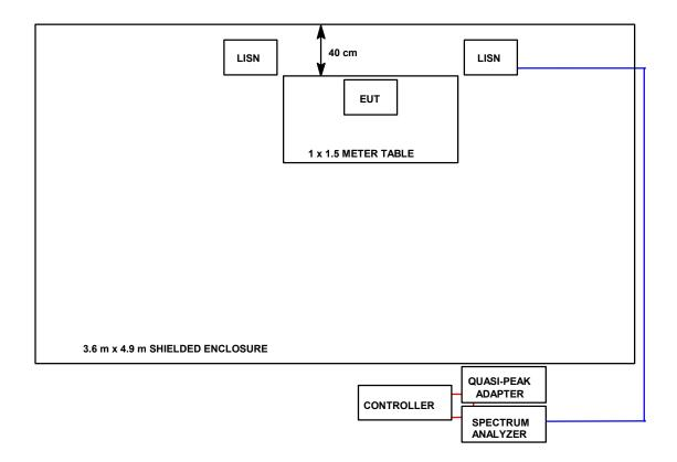
FIGURE 2: Radiated Emissions Test Setup
