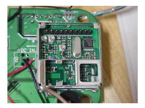
Front View of Infrared Sensor PCB
