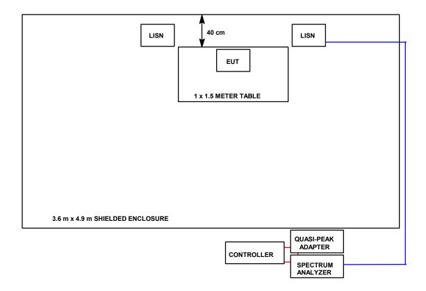
FIGURE 2: Radiated Emissions Test Setup
