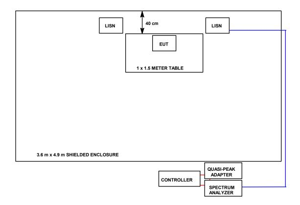
FIGURE 2: Radiated Emissions Test Setup
