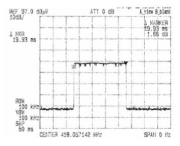
Note: Maximum duty cycle cover letter states maximum duty cycle to be 23.3 mS with encrypted packet.
