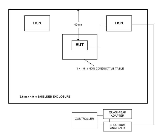
FIGURE 2: Radiated Emissions Test Setup
