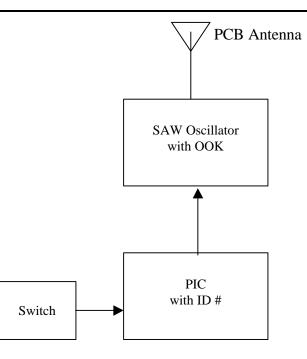
BLOCK DIAGRAM Core Technology 418 MHz Home Security Transmitter Door/Window Sensor Model Number XDS125
