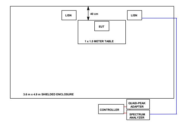
FIGURE 2: Radiated Emissions Test Setup
