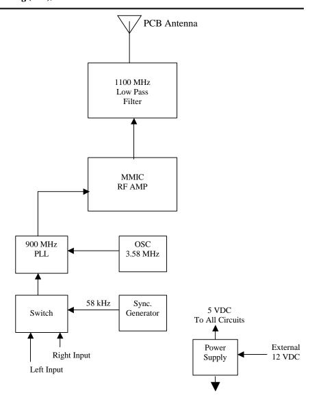
BLOCK DIAGRAM Core Technology Wireless Speakers Transmitter Model Number WS920
