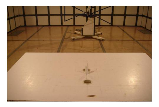
**Radiation Emission Test View For 1GHz-25GHz**
