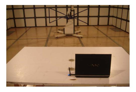
**Radiation Emission Test View For 1GHz-25GHz**
