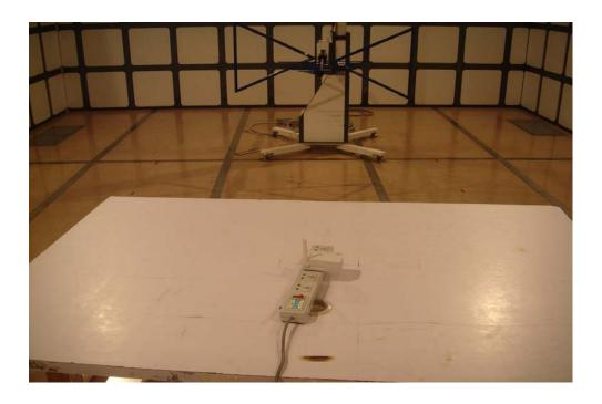
**Radiation Emission Test View For 1GHz-25GHz**
