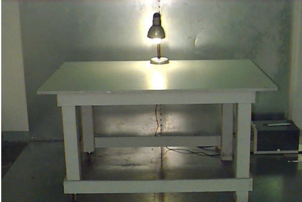
Maximized Conducted Emissions Test Set-up – Front View
