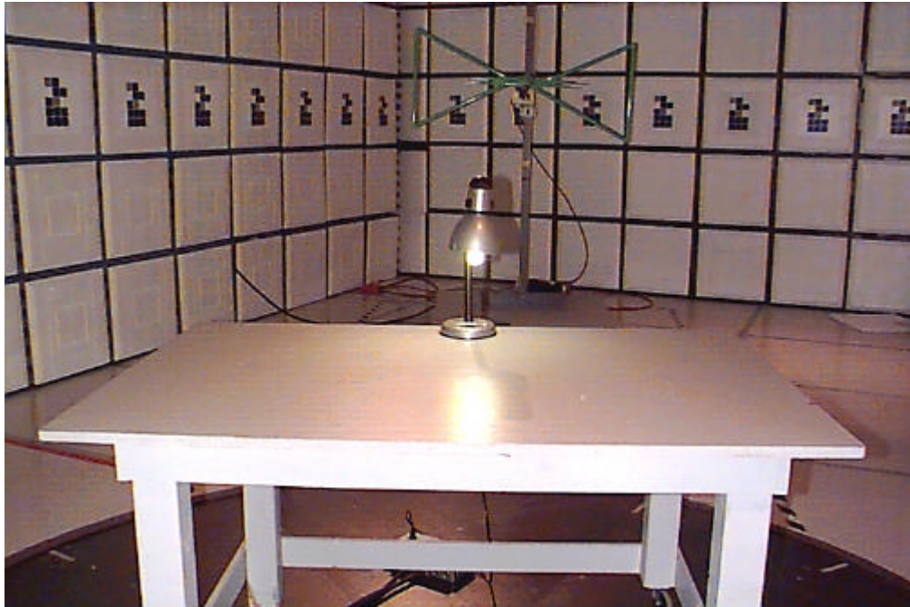
Maximized Radiated Emissions Test Set-up – Front View
