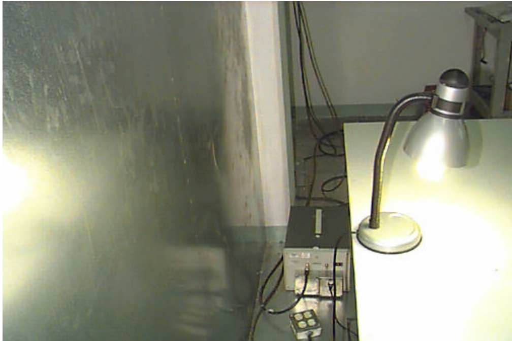
Maximized Conducted Emission Test Set-up – Rear View
