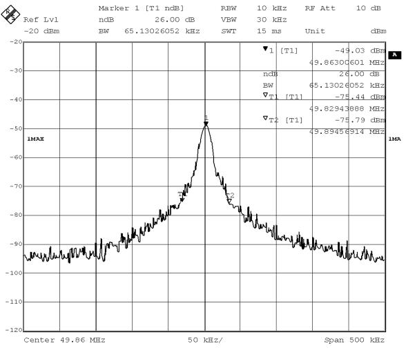
26dB bandwidth lower frequency :49.82943888MHz 26dB bandwidth upper frequency :49.89456914MHz
