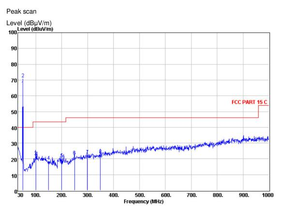
**30 MHz~1 GHz Field Strength of Unwanted Emissions.Quasi-Peak Measurement** Vertical:
