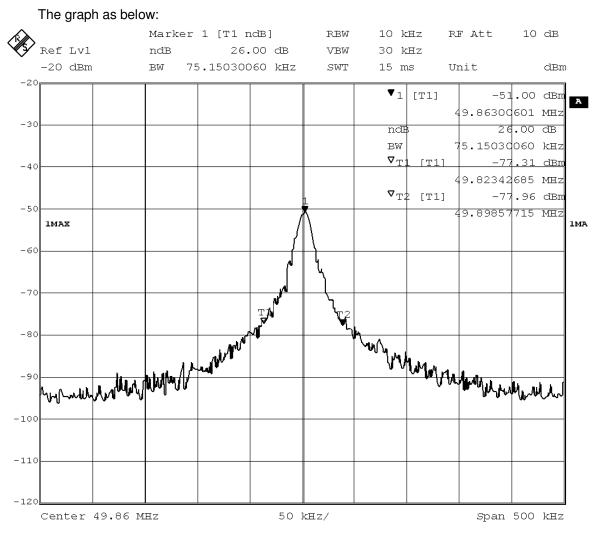
26dB bandwidth lower frequency :49.82342685MHz 26dB bandwidth upper frequency :49.89857715MHz
