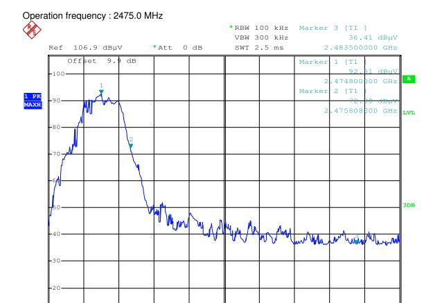
According to above plot, 20dB bandwidth falls in assigned band (2400-2483.5)MHz. It is deemed to comply with section 15.215
