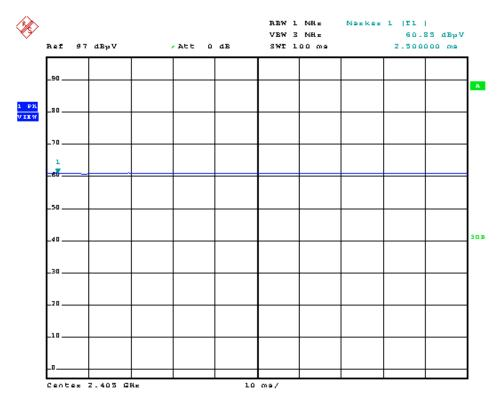
According to above plot, the duty cycle of the this device is 100%, plused operation according to C63.10 clause 7.5 is not employed and the average correction calculation is not applied on this report.
